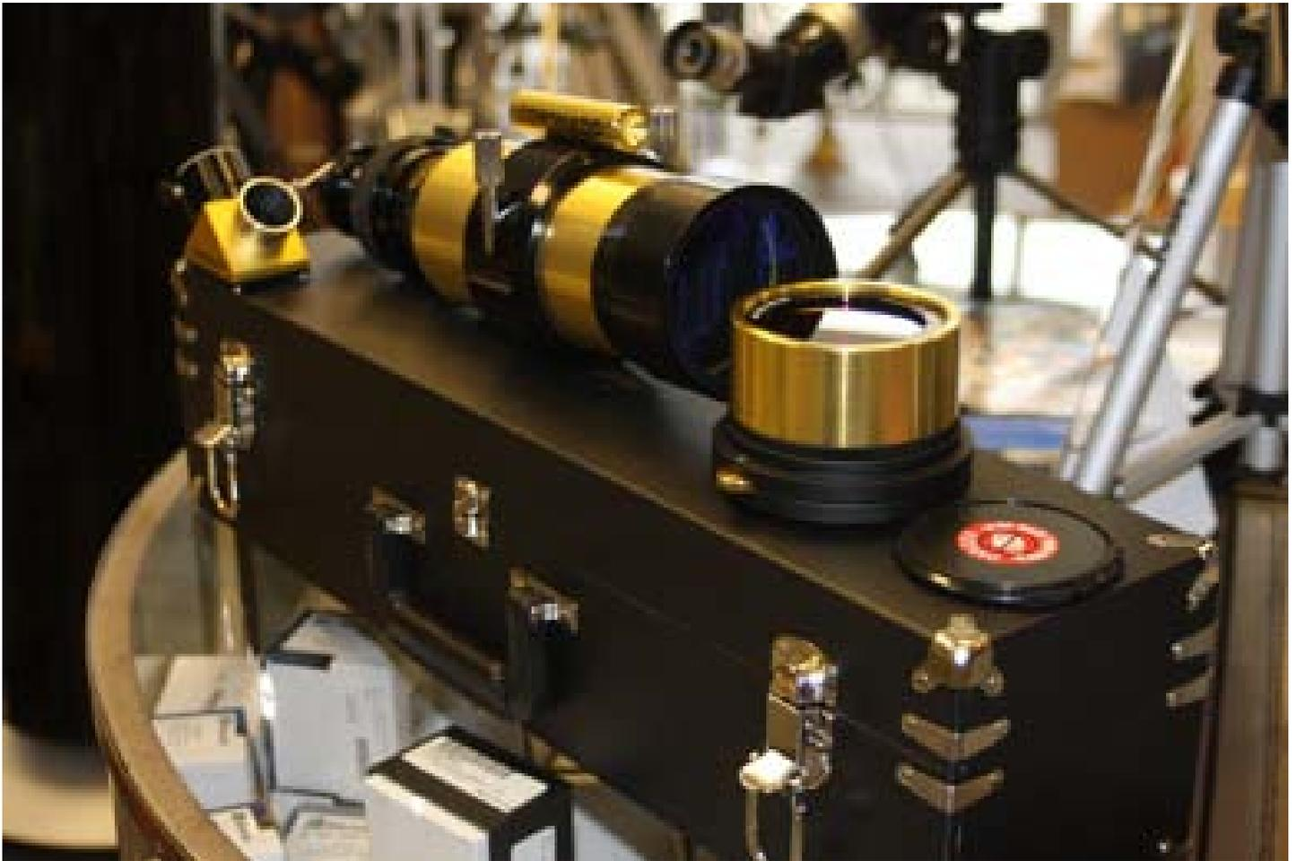
The 60mm etalon was attached to a T-max tuner and screwed into the end of the telescope in front of the clear blue objective. There was an empty gold tube that led to an ERF inside the scope and then to a 2 inch helical focuser which held a 1.25 inch drawtube containing a BF10 Blocking filter encased inside a 1.25 inch star diagonal. There was a plastic clip on etalon cover and a white eyepiece plug in the diagonal.
