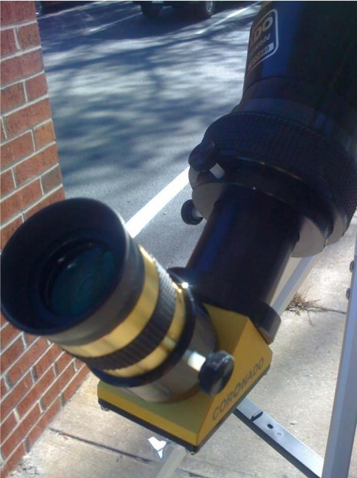
The Coronado Maxscope 60 has the same aluminum drawtube/ Helical focuser that is on all of the MaxScopes. I am personally not a big fan of this system as it is not very strong and has no way to lock the focus in place.
