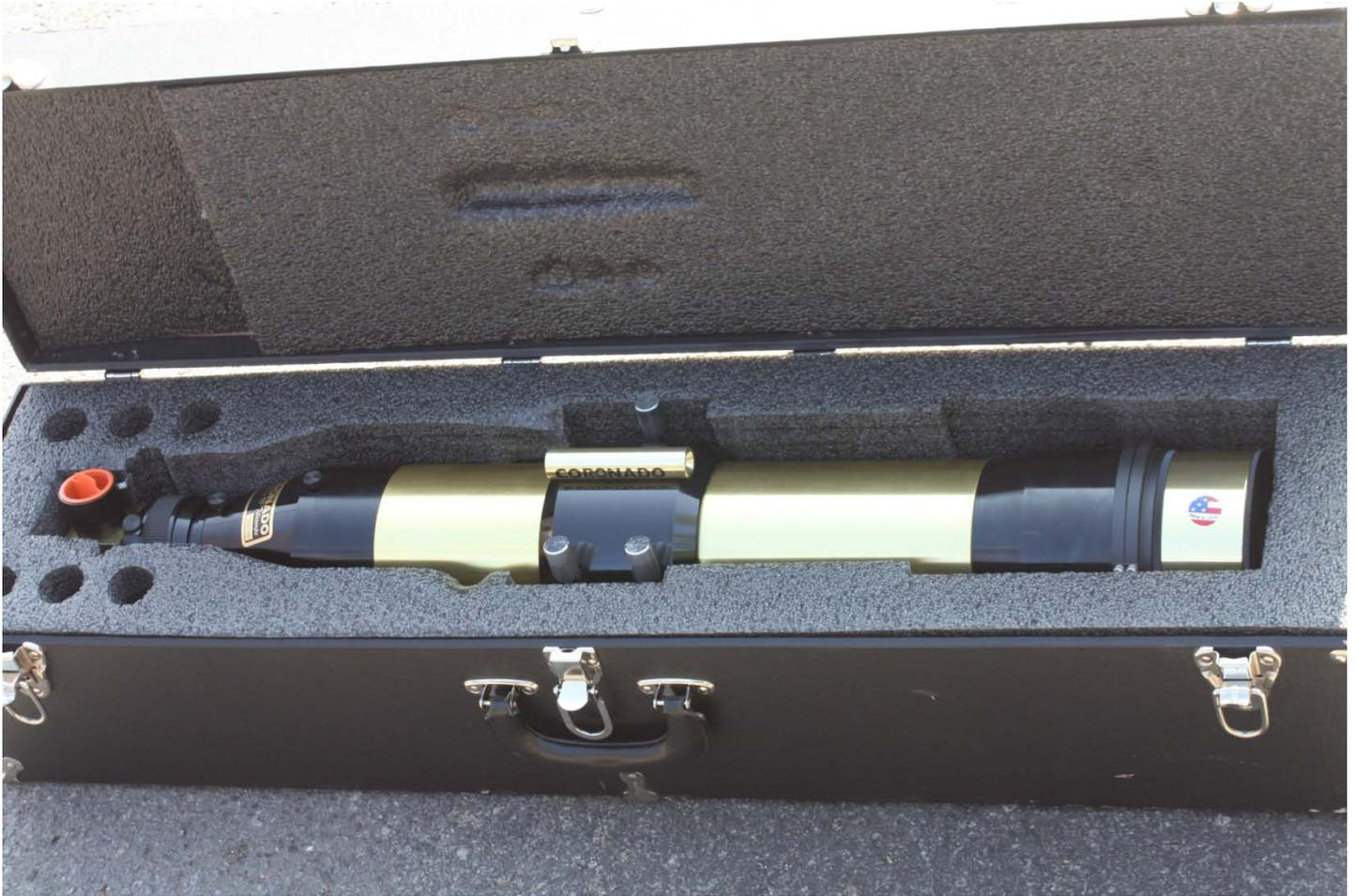
The included SolRanger sunfinder is a big plus. It is very sturdy and is aligned perfectly with the scope by use of predrilled holes in the clamshell. It is awesome.
