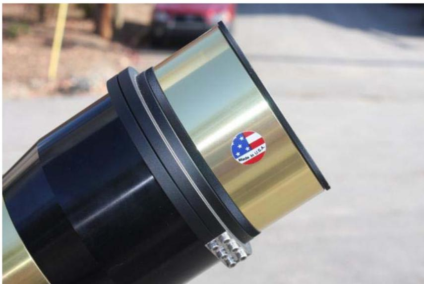
The entire etalon assembly tilts with this wheel as shown in the picture to the left.
