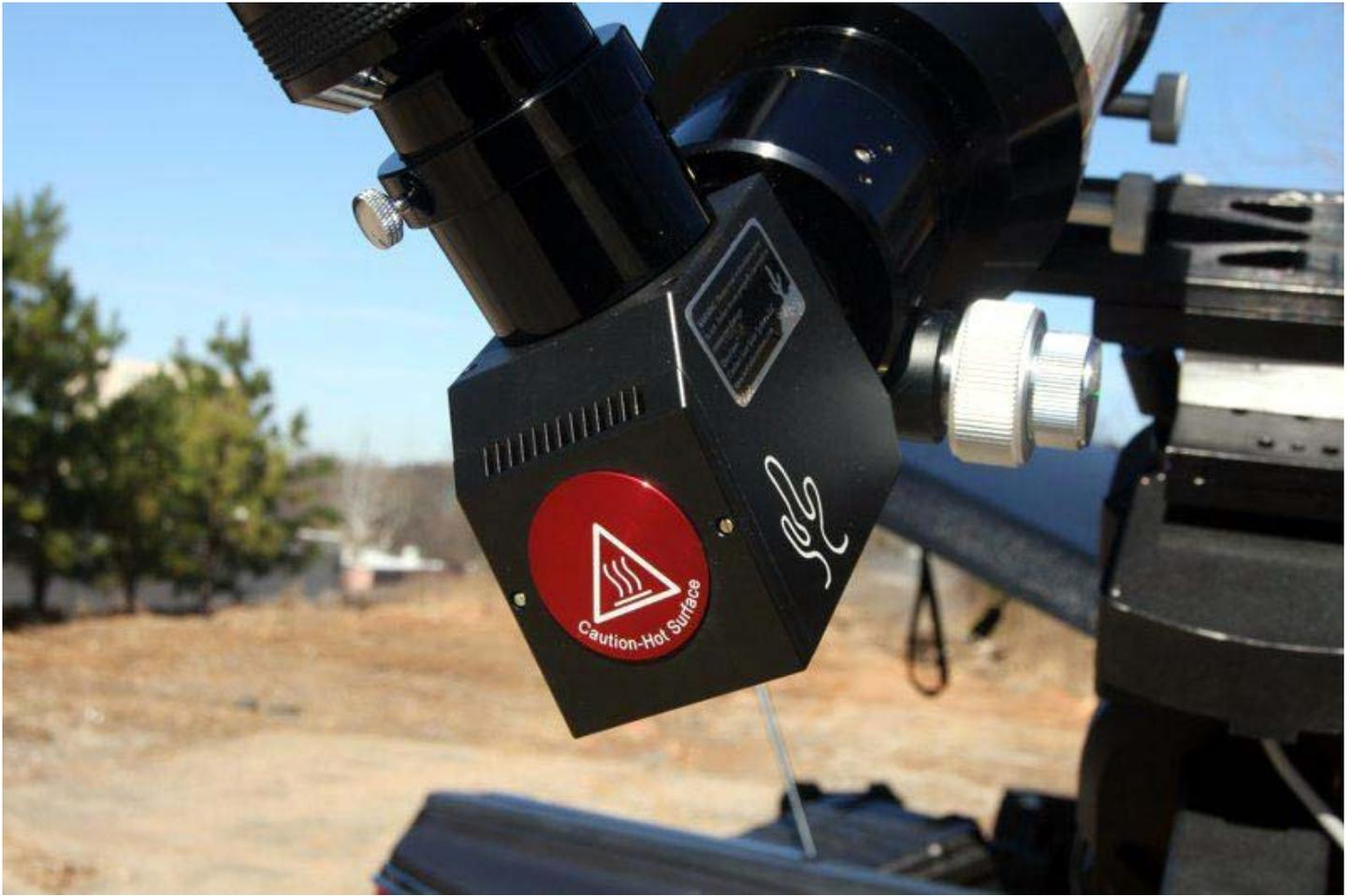
I attached the wedge to a 127mm Explore Scientific refractor mounted to a Celestron CGE mount on a Pinnacle Portable pier. I screwed the polarizers onto the bottom of a William Optics 28mm UWAN 2 inch eyepiece and inserted them into the wedge.
