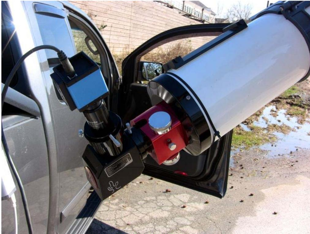
The image was astoundingly clear and very detailed through the camera. I was extremely impressed with the ease of use. The polarizers were not necessary as I used the green #58 filter again. I did try a Meade polarizer in between the camera and wedge but it extended the focal length too far to focus so I just took it out. I tried the camera with a 2X, 3X and a 5X Barlow lens and was able to focus and get a decent image with all Barlows.
